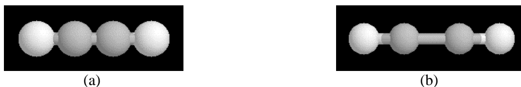
Figure 3.2: Animation of C\equiv C stretching mode in acetylene. Weighted eigenvectors are added to its original coordinates to visualize compression and extension of C \equiv C bond in (a) and (b), respectively.
